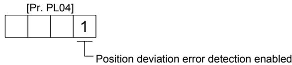
When you compare the model feedback position ( 1)) and the feedback position ( 2)) in figure 15.1, if the deviation is more than the value of [Pr. PL05 Position deviation error detection level] (1 mm to 1000 mm), [AL. 42.1 Servo control error by position deviation] will occur and the linear servo motor will stop. The initial value of this detection level is 50 mm. Change the set value as necessary.
