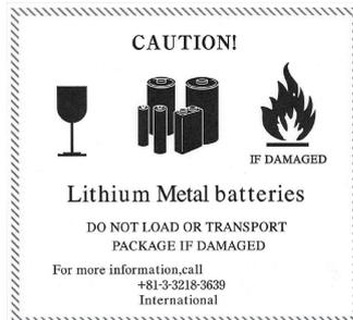
Figure. Example of Mitsubishi Label with Battery Illustration
